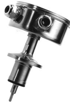
ø80 mm housing with 2 glands Cover not mounted 3A/DN38 connection at the rear Fast response sensor
